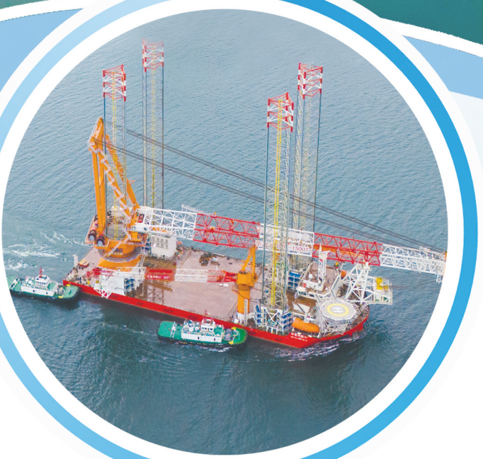
“华夏鸿鹄01”自升自航式风电安装船
